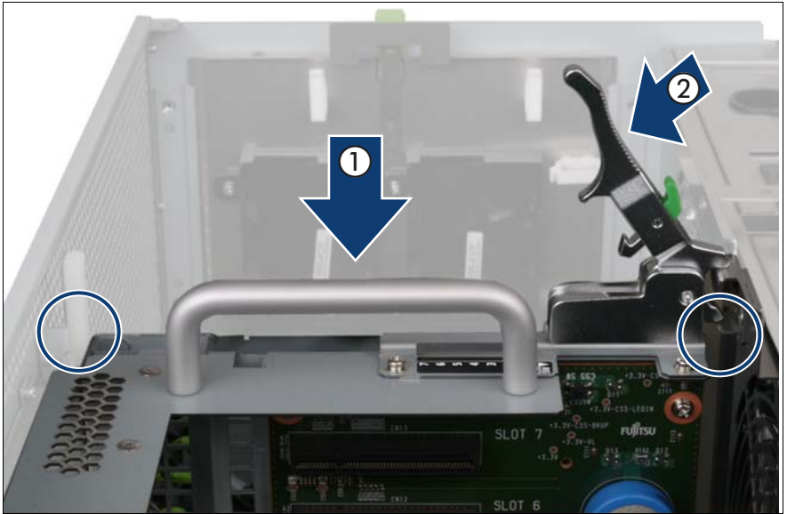
Figure 89: Installing the PCI Riser
